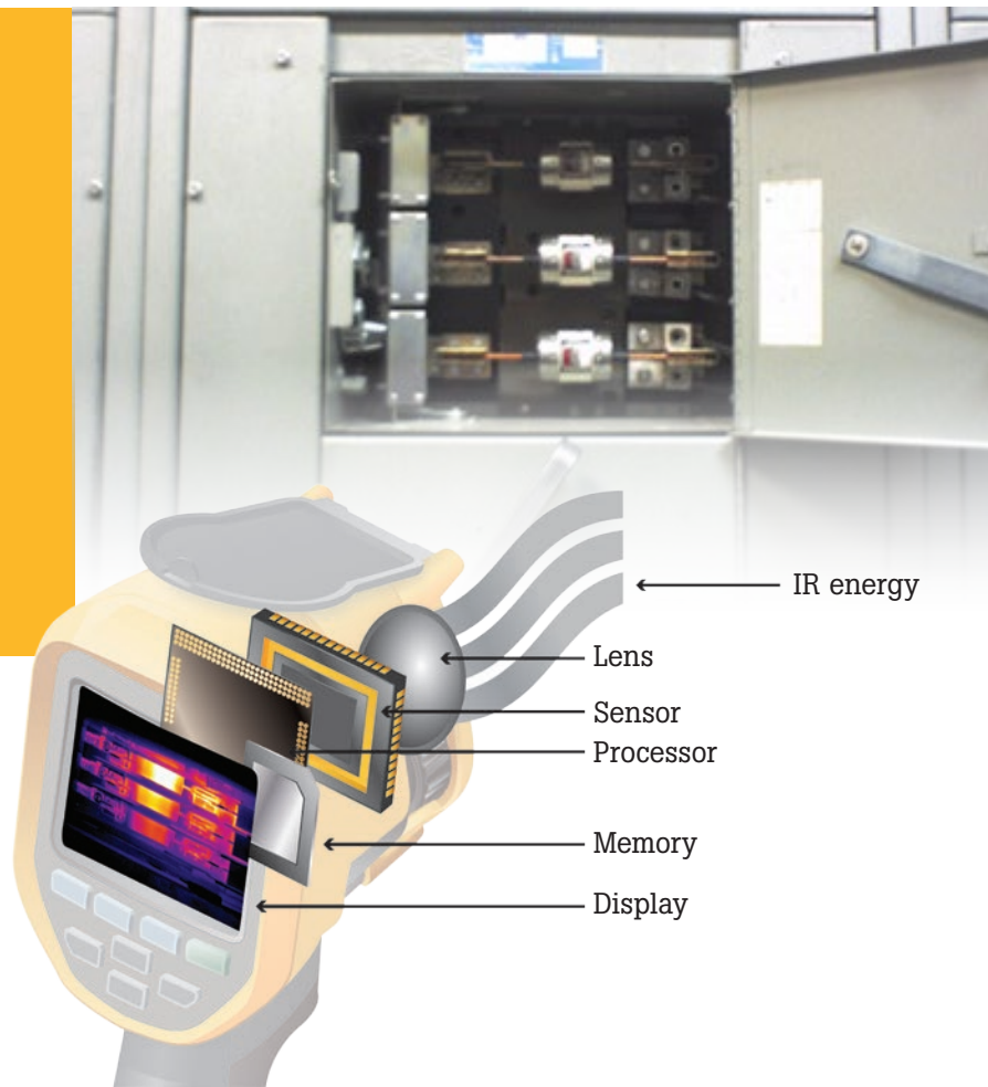
Figure 1. Anatomy of an infrared camera
