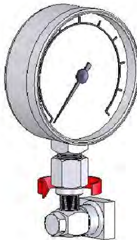
Figure 2. Connect Assembly to Test Port
