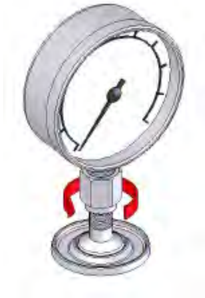
Figure 2-2. Connect Assembly to Test Port
