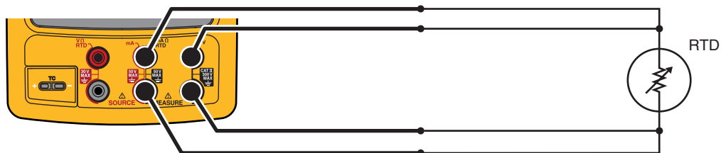
Figure 17. Temperature Measurement with an RTD
