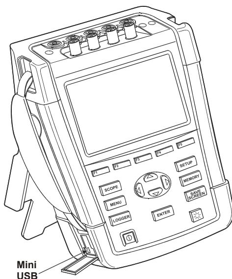
Figure 4-1. Tilt stand and location of USB interface connector
