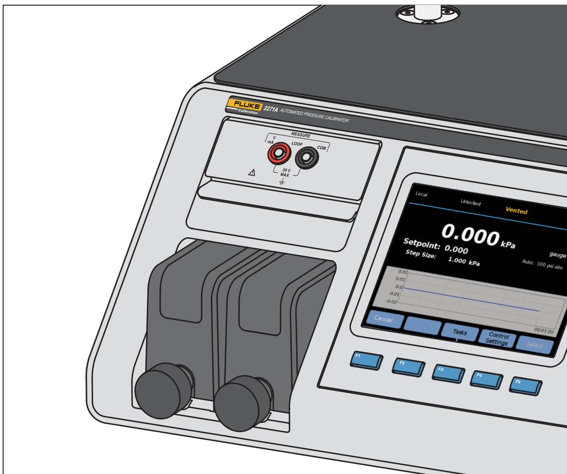
Figure 3. Installed EMM and PMM Modules
